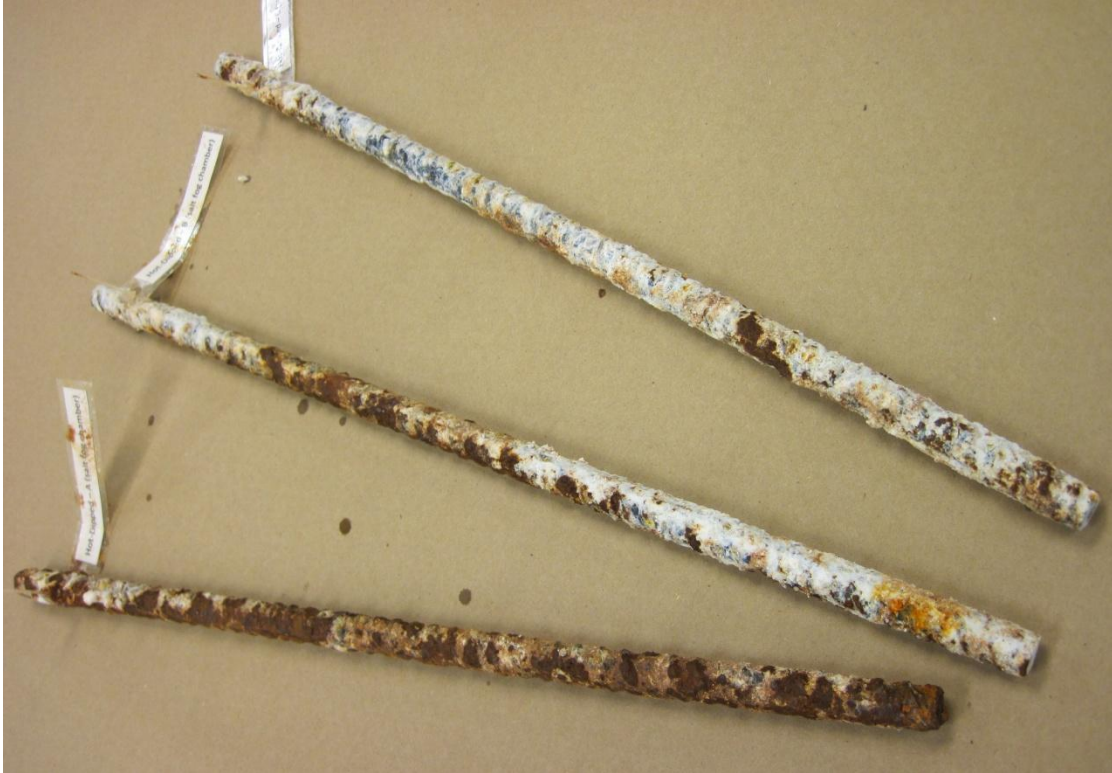
Figure 3 Traditional Hot Dipped galvanizing after 3000 hours in salt fog exposure
