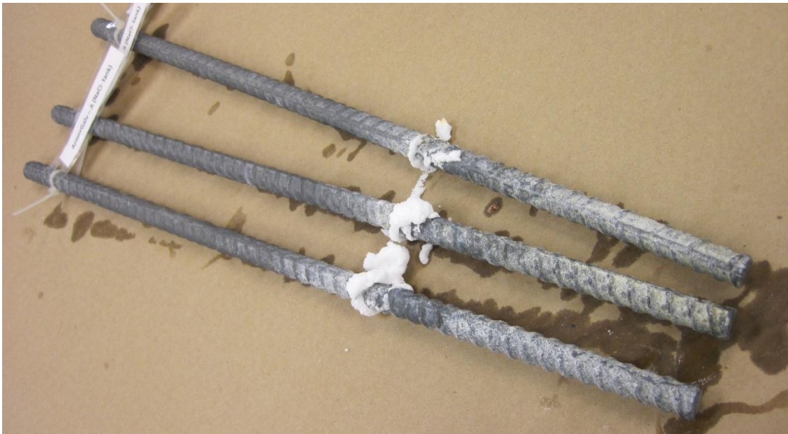
Figure 2 Armorgalv ® process after 3700 hours of partial immersion
