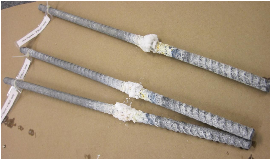
Figure 1 Traditional Hot Dipped galvanizing after 3700 hours partial immersion
